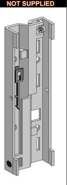
The placement of the bracket on the rear of the loudspeaker detemines the angle between the loudspeaker and the wall.
